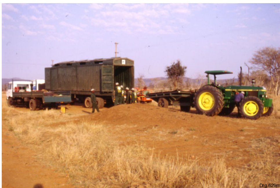
Figure 11 — Elephant recovery to a family crate using a tipping trailer
